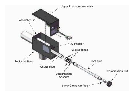
Figure 2: Mast3rPur System Exploded View
