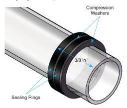
Figure 3: Quartz Tube Seal Assembly Detail
