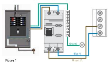
**Optional 1:** Dual Service, TN and TT Electrical Systems (2x16 Amp). 5 Wires (2 Lines + 2 Neutrals + 1 Protective Earth)\*. Protective Earth wire (Green/Yellow) must be connected to system ground terminal as marked. The heater runs on service line L1. All equipment (pumps, etc.) runs on service line L2.
